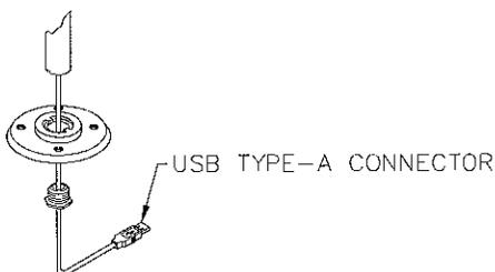
Thread the TYPE-A connector through a hole in the mounting surface and conduit nipple, or breakout one of the tabs in the surface mount plate (use wide, square jaw pliers) and route the cable through the conduit nipple. Thread the cable through the surface mount plate and pole. Holding the pole in the plate, tighten the conduit nipple into the pole. Attach the mounting plate to the surface, being careful to route the cables through the breakout tab if applicable
