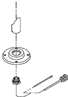
Thread the DIN8F connector through a hole in the mounting surface and conduit nipple, or breakout one of the tabs in the surface mount plate (use wide, square jaw pliers) and route the cable through the conduit nipple. Thread the cable through the surface mount plate and pole. Holding the pole in the plate, tighten the conduit nipple into the pole. Attach the mounting plate to the surface being careful to route the cables through the breakout tab if applicable
